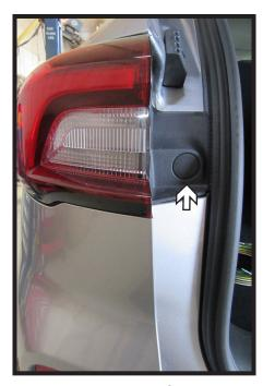
Remove the bolt cover from the tail light housing. Do this on both sides of the vehicle.
