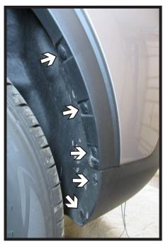
2. Remove the five (5) push pins from along the edge of the rear wheel well. Do this on both sides of the vehicle.
