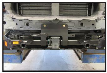
19. Reinstall the four (4) bolts attaching the ACC to the frame.
