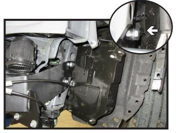
23. Reinstall the black box onto the driver side of the vehicle. Reattach the wire loom to the bottom bolt on the backside. If the box touches the baseplate bolt head, bend back plate slightly to create clearance (inset).
