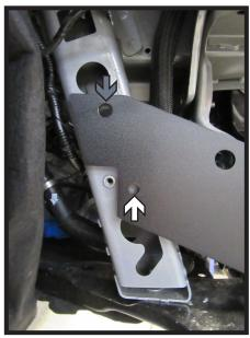
16. Using a 3/8" drill bit, drill out the back bottom hole (white) using the baseplate as a template. If needed use a 1/2" drill bit, drill out the back top hole (gray). Do this on both sides of the vehicle.
