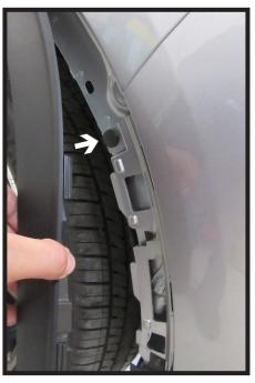
Pull back the wheel well trim and hold in place with a soft cloth. Remove the one (1) push pin from the rear panel joint. Do this on both sides of the vehicle.
