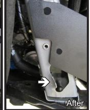
17. Using a pair of large vise grips bend back the frame piece as shown to create an access hole for the nut plate. Do this on both sides of the vehicle.
