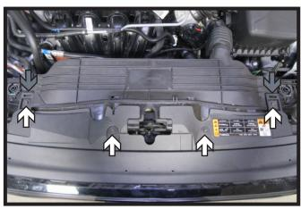
Using a 10MM socket, remove the four (4) bolts (white) from the top edge of the fascia. There are two (2) on each side. Then unclip the two (2) push pins (gray), one (1) on each side.
