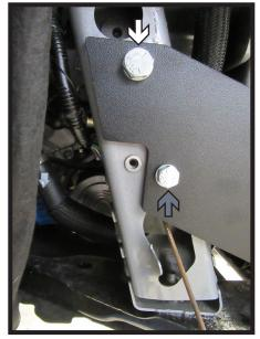
18. Insert nut plate through hole in the frame. Insert a 1/2" bolt with lock washer into the top hole (white) and a 3/8" bolt with lock washer into the bottom hole (gray). Do this on both sides of the vehicle.
