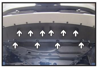
5. Using a T30 Torx, remove the ten (10) bolts from the bottom of the fascia.
