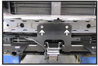
15. Install two (2) 1/2" bolts with washers and wire nuts. Torque bolts to 50 ft/lbs.
