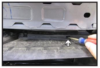
11. Remove the shroud around the lower shutters by removing the two (2) push pins, one (1) on each side of the vehicle. Then using a flat screw driver, remove the eight (8) clips around the edge of the shroud. The shroud will not be reinstalled.
