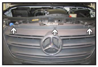
1. Using a T25 Torx, remove the three (3) bolts from the top of the fascia.
