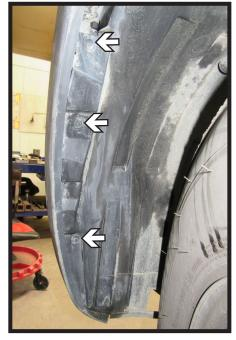
2. Remove the three (3) push pins from along the edge of the wheel well. Do this on both sides of the vehicle.
