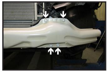
8. Using a 13MM socket, remove the four (4) bolts from each side of the bumper. Unclip the wire loom from the back of bumper as it is removed. Set bumper aside to be reinstalled later.
