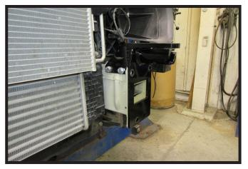
Remove the three (3) bolts from the front of the baseplate. Do this on both sides of the vehicle.
