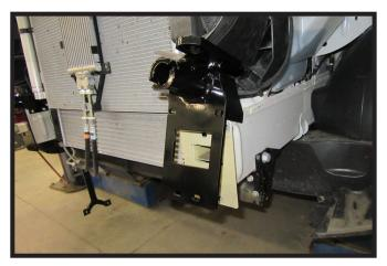
11. Tip baseplate upward and slide onto the frame of the baseplate.
