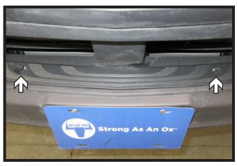
3. Using a T45 Torx, remove the two (2) bolts from the fascia, above the licence plate holder.
