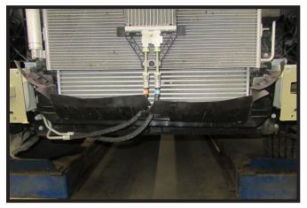
9. Unsnap and remove the plastic shroud from the bottom of the radiator.
