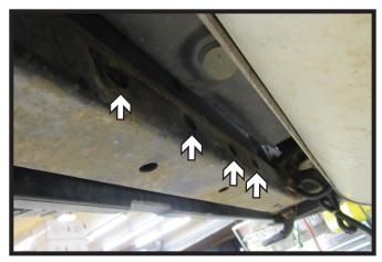
2. **Mopar Off-Road Bumper**: Using an 18MM socket, remove the four (4) existing bolts and spacer plate (located between bumper and cross member). The spacer plate will not be reinstalled. Then slide the receiver hitch onto the cross member so the four (4) holes on the hitch line up with the holes on the cross member.
