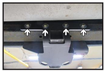
Install four (4) 1/2" bolts from the back side of the cross member with flat washers and whiz nuts.
