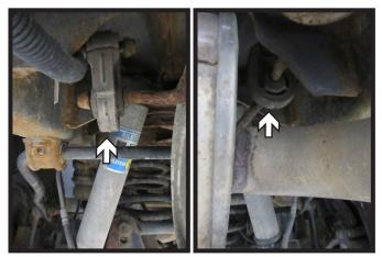
Standard Models: Support exhaust and remove rubber isolator from exhaust rod on each sides of the vehicle (above). Lower the exhaust to allow for easier receiver hitch installation. Note: This can be done using Exhaust
