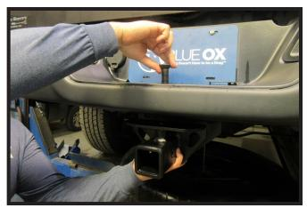
3. Raise hitch into position and start the hex drive flat head screw in to hitch ball hole. Hand tighten at this time.
