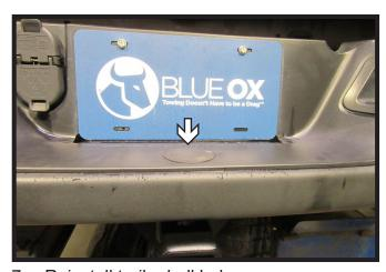
7. Reinstall trailer ball hole cap.
