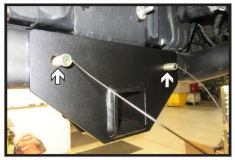
5. Pull bolts and spacer plates through vehicle into position as shown.
