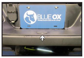
2. Remove the trailer ball hole cap for the center of the bumper.
