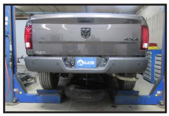
1. If needed, lower spare tire to allow for easier installation.
