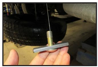
4. Feed lead wire through rear cross member. Slide spacer plate onto 1/2" bolts and attach lead wire to end of bolt. Do this on both sides of the hitch.
