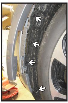
4. Remove the four (4) push pins from along the edge of the wheel well. Do this on both sides of the vehicle.
