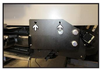
22. Using a 3/8" drill bit, drill out the two(2) holes in the top bumper using the baseplate as a template. Do this on both sides of the vehicle.
