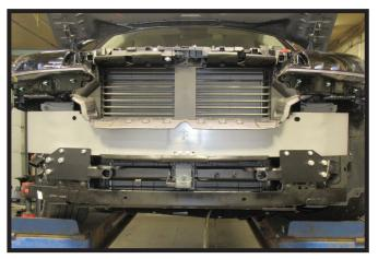
24. Reinstall bottom bumper with existing nuts and bolts.
