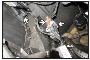
9. Lift up on the tabs on top of the fascia and start to remove. As the fascia is removed, unplug the three (3) electrical connections on the passenger side of the vehicle. Remove fascia and set aside to be reinstalled later.
