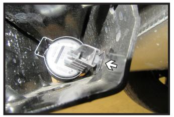
2. Unclip and remove electrical plug from bracket. Let hang.
