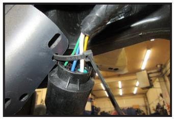
3. If present, zip tie electrical plug to passenger side of the receiver hitch as shown.
