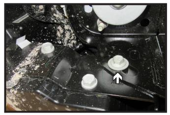
5. Using a 13MM socket, remove the one (1) bolt from the back of the bumper on the driver side of the vehicle. Then loosen the same bolt on the passenger side of the vehicle. Open rear door and pull bumper away from the vehicle slightly.
