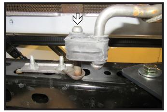
1. Remove rubber isolator from exhaust rod on each side of the vehicle. Lower exhaust.
