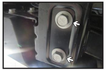
4. Using a 18MM socket, remove the two (2) bolts from behind the bumper. Do this on both sides of the vehicle.
