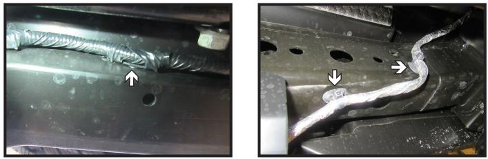
1. Unclip the wiring loom from the bumper and frame on the driver side of the vehicle. Let hang.
