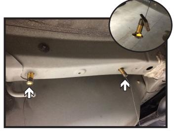
5. Feed lead wire from furthest existing frame hole to the access hole. Place spacer plates onto wire then attach lead wire to the end of the 1/2" carriage bolt (inset). Pull bolt and spacer plate through the frame. Repeat process with second bolt hole. Ensure spacer plates are sitting flush against inner frame and the bolts are hanging vertically. Do this on both sides of the vehicle.
