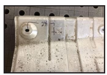
6. Measure 2-3/4" from the forward existing hole in the heat shield. Using a 1-1/2" hole saw, drill a hole in the heat shield in line with the existing holes. Repeat this step on second heat shield if present.
