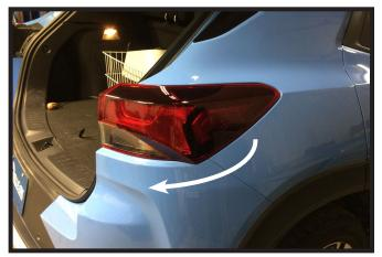
3. Push tail light toward the rear, remove and let hang. Do this on both sides of the vehicle.
