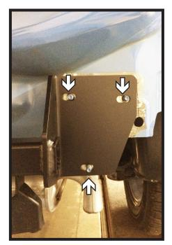
19. Slide the receiver onto the vehicle. Apply clear 100% silicone around the three (3) bolt holes of the receiver. Do this on both sides of the vehicle.
