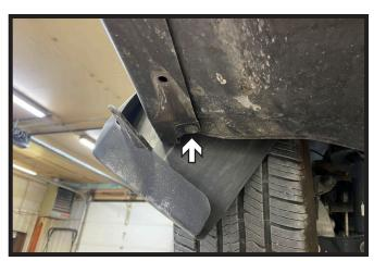
Rotate mud flap outward and remove the one (1) push pin from behind the wheel on the driver side of the vehicle. Remove plastic cover on driver side and set aside to be reinstalled later.
