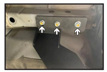
11. Raise hitch into position. Remove lead wires and loosely install 1/2" whiz flange nut onto each bolt. Do this on both sides of the vehicle. Then tighten all bolts.
