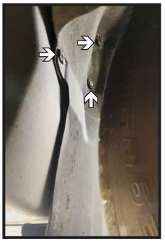
5. Remove the three (3) push pins from behind the tire on the driver side of the vehicle.
