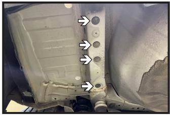
7. Remove the four (4) rubber plugs from the bottom of the frame. Do this on both sides of the vehicle.
