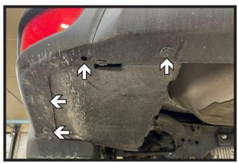
4. Remove the four (4) push pins from the underside of the vehicle on the driver side.
