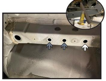
9. Starting with the rear hole, run a lead wire from the rear hole (white) to the access hole. Place a spacer plate onto the wire then attach the lead wire to the end of the 1/2" carriage bolt (inset). Pull bolt through the frame. Ensure the spacer plate is sitting flush against inner frame and the bolt is hanging vertically. Do this for the remaining two (2) holes (gray). Do this on both sides of the vehicle.
