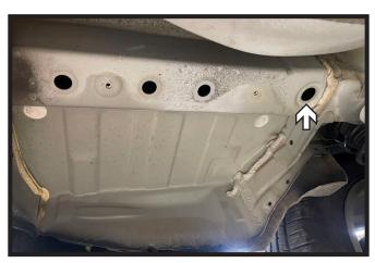
8. Using a 1-1/4" hole saw, drill out the forward most hole to create an access hole. Do this on both sides of the vehicle.
