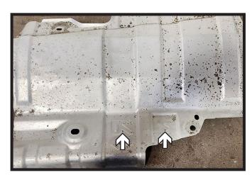
10. **Optional**: Using a 5/8" drill bit, drill out the two (2) dimples in the heat shield and reinstall on the passenger side of the vehicle using existing hardware.
