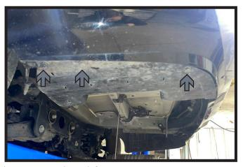
4. Remove the two (2) screws (white) and three (3) push pins (gray) from the plastic cover on the driver side of the vehicle. Remove cover and set aside to be reinstalled later.
