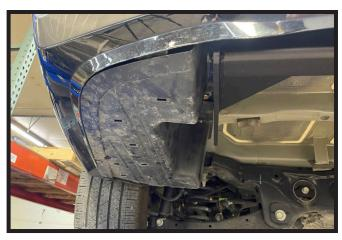
Reinstall plastic cover on the driver side of the vehicle.
