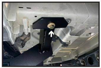
7. Raise the receiver hitch into place and start the one (1) M12 bolt with conical washer into the bottom hole. Ensure the teeth of the conical washer are towards the hitch. Do this on both sides of the vehicle.
