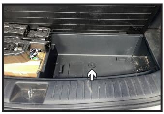
Open lift gate of the vehicle. Pull up on the tab to bottom compartment and remove the roadside assistance tool insert. Unscrew the cap in the bottom to access the nut holding the spare tire in place.
