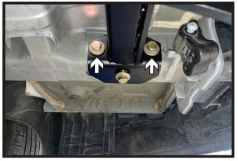
8. Start the two (2) M12 bolts with conical washers into the side holes. Ensure the teeth of the conical washers are towards the hitch. Tighten bottom bolt then tighten side bolts. Do this on both sides of the vehicle.
