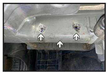
5. Remove the three (3) stickers covering the bolt holes needed to attache the receiver hitch to the frame. Do this on both sides of the vehicle.
