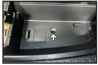
Using the wrench provided with the roadside assistance tools let down the spare tire to allow clearance for receiver hitch installation.
