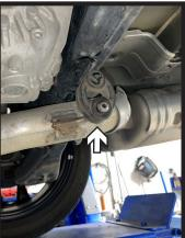
3. Support exhaust using a jack or stand. Remove the four (4) rubber isolators from the exhaust rods on the passenger side of vehicle. If vehicle is equipped with dual exhaust, repeat step on the driver side of the vehicle. Lower exhaust(s) to allow for receiver hitch installation.
