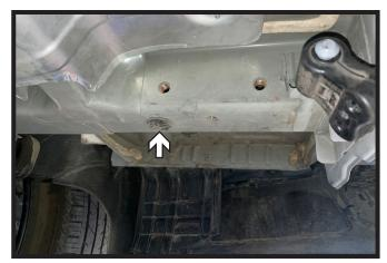
Remove the rubber plug on the bottom of the frame to allow for receiver hitch clearance. Do this on both sides of the vehicle.
