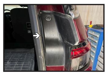
7. Using a flat screw driver, remove the plastic piece next to the tail light. Set aside to be reinstalled later. Do this on both sides of the vehicle.
