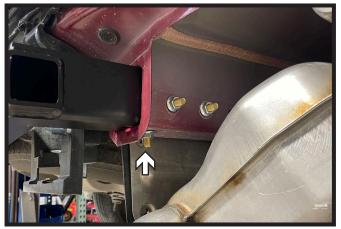
14. Start the one (1) 1/2" carriage bolt in the front bottom frame hole. Do this on both sides of the vehicle.
