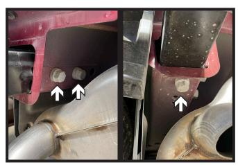
12. Using a 21MM socket, remove the three (3) bolts from the rear bumper. There are two (2) on the side and one (1) on the bottom. Do this on both sides of the vehicle. Remove rear bumper, it will not be reinstalled
