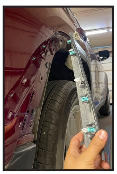
3. Pull back the wheel well trim, releasing the push pins, past the fascia joint. Prop trim away from the vehicle using a soft cloth. Do this on both sides of the vehicle.
