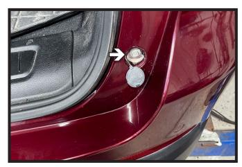
Using a 10MM socket, remove the one
