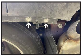
Using a 10MM socket, remove the two (2) bolts from the bottom of the rear fascia. Do this on both sides of the vehicle.
