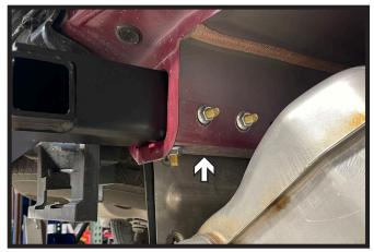
15. **Non-L Models**: Start the 5/16" carriage bolt with lock nut in the bottom rear hole of the frame. Do this on both sides of the vehicle. Tighten all bolts at this time.
