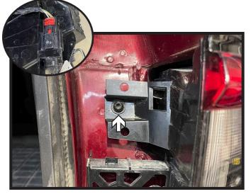
Using a T30 Torx, remove the bolt next to the tail light. As the tail light is removed, unplug electrical connection (inset) on the back of the light. Set tail light aside to be reinstalled later. Do this on both sides of the vehicle.
