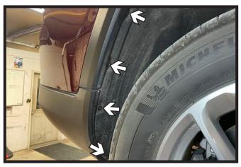
Using an 8MM socket, remove the four (4) bolts from along the edge of the rear wheel well. Do this on both sides of the vehicle.
