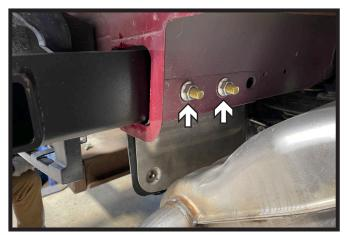
13. Clean out any road debris from inside of the frame on both sides of the vehicle. Slide the receiver hitch into the frame. Start two (2) 1/2" carriage bolts with flat washers and lock nuts in the side frame holes. Do this on both sides of the vehicle. L Models: Use the set of holes farthest from the hitch cross bar.
