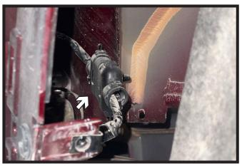
5. Unclip the electrical connection from behind the rear tire. Do this on both sides of the vehicle.
