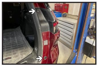
6. Lift tailgate. Using a flat screw driver, remove the two (2) plastic covers next to the tail light. Do this on both sides of the vehicle.
