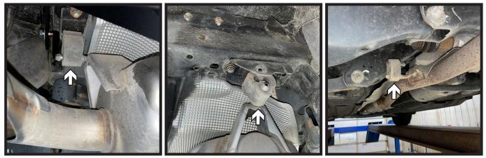
1. Support exhaust using a jack or stand. Remove the three (3) rubber isolators from the exhaust rods, there is one (1) on each side of the vehicle and one (1) towards the front. Lower exhaust to allow for receiver hitch installation.
