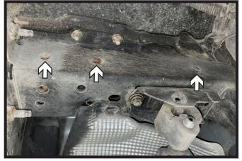
2. Clean road debris out of existing bolt holes. Then run a M12 x 1.25 tap through the holes. Verify that the provided 12MM bolts will fit in the holes after they have been cleaned. Do this on both sides of the vehicle.
